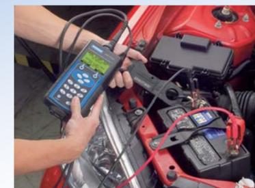
Using the optional Amp Clamp provides an enhanced level of diagnostics beyond just starter voltage drop. The EXP starter diagnostics include starter amps draw, voltage drop, start time, and starter circuit resistance resulting in more accurate results.
